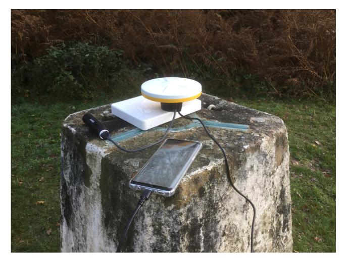
A basic GPS receiver like this costs around £300. You can buy them off the shelf or make your own. (See the reference material below.) To keep the cost down many receivers use a nearby smartphone to provide a display, signal processing and Internet access.
